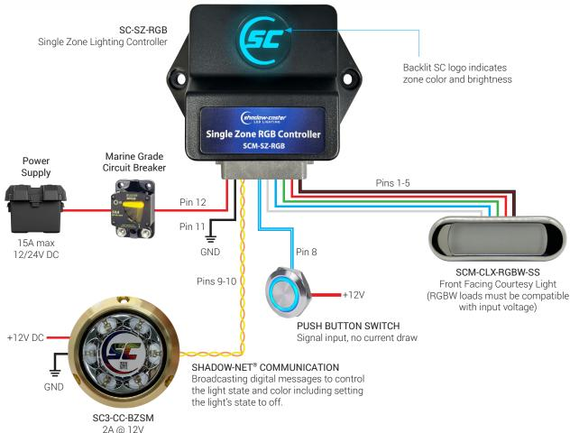
**Note:** Shadow-NET current draw does not add to the 10A budget for the Single Zone Controller
