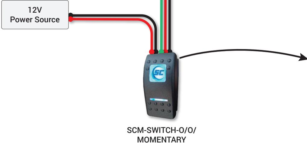
Shadow-NET wires are not connected when using a switch.
