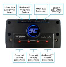
The Light Commander has four built in RGBW channels. By default these RGBW channels correspond to zones 1-4, identified in the device list as "LOCAL 1-4" (see Configure Devices screen shot on page 11). However, they are independent and can be assigned to any of the configured zones 1-6 supported by the controller.
