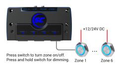
There is one global control input, that will step between colors on subsequent presses.
